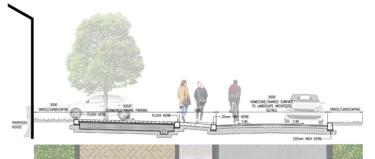
Figure 79. Secondary road cross-section exemplifying horizontal arrangements and materialisation of streets in the scheme. Source: MCORM, 2022.
