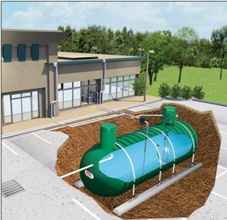
Plate 2-1. Example of Rainwater Harvesting System
