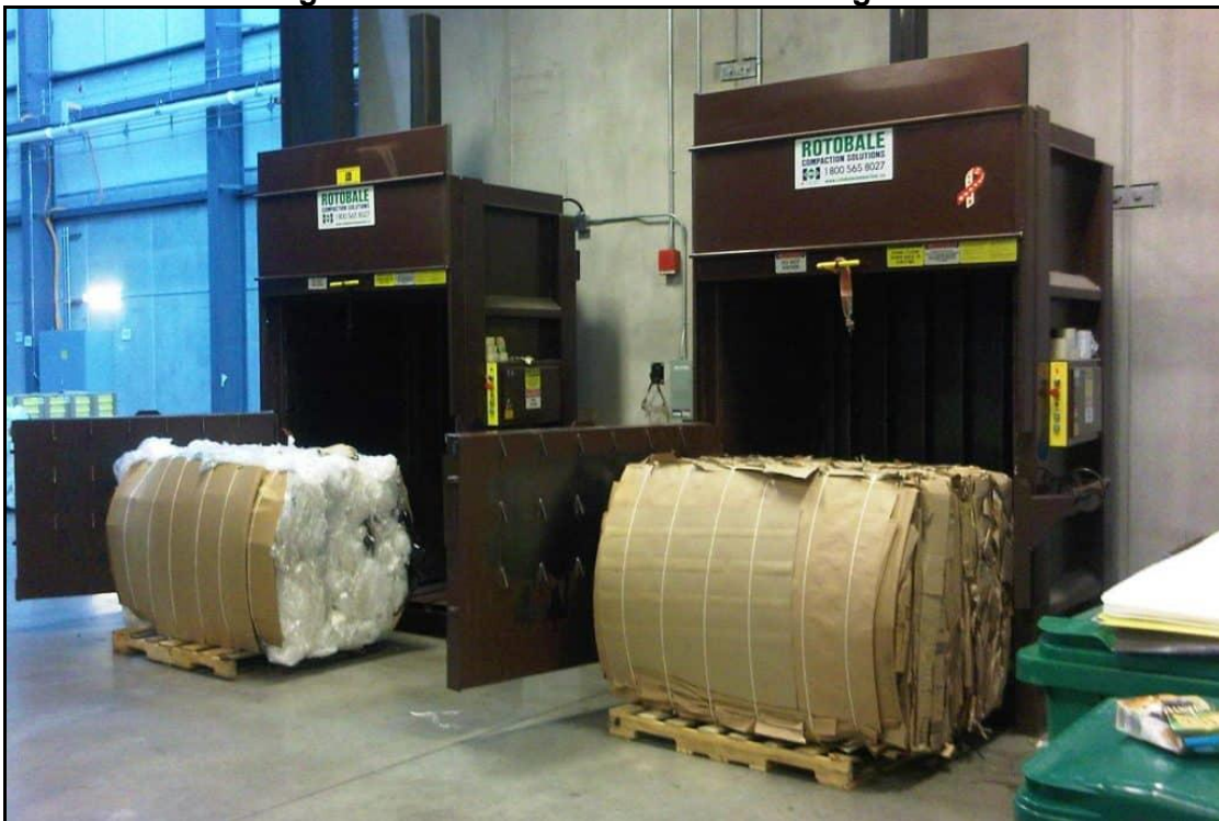
Figure 4 Cardboard/Plastic Bailing Units
