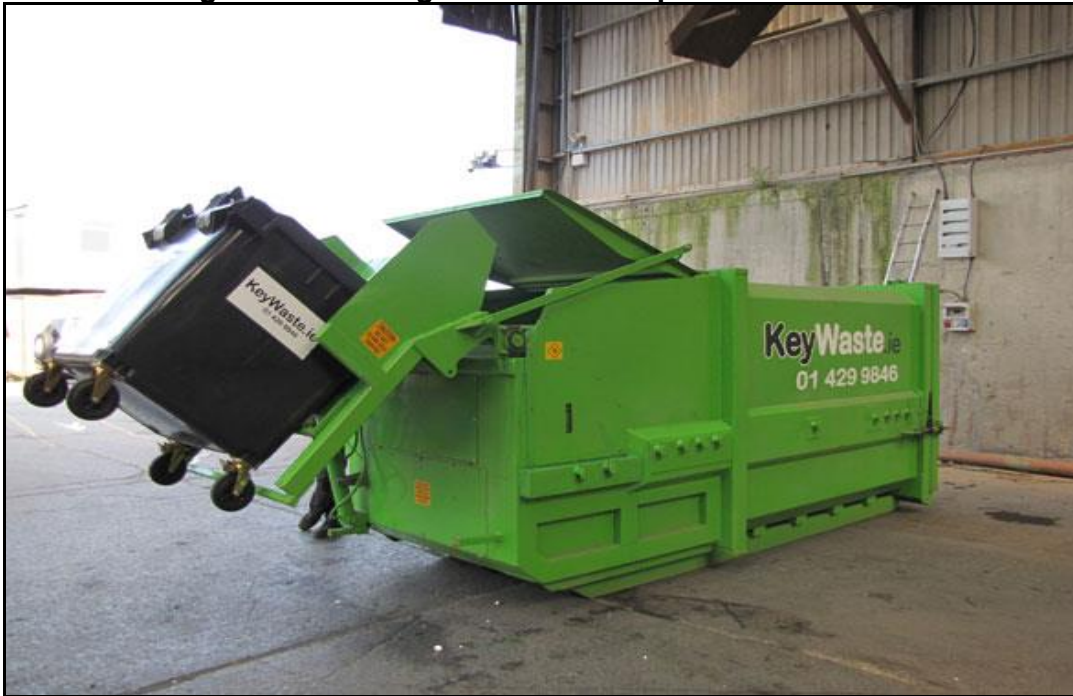
Figure 3 Image of mobile compactor with bin lift
